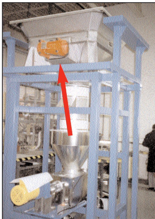
SCR-300 on Box Dumper to prevent hang-ups.
