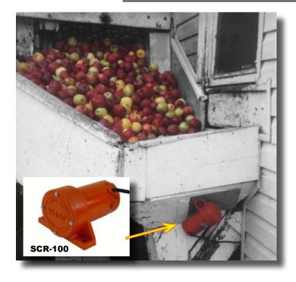
An apple orchard was experiencing problems with apples not feeding properly through a hopper to the entrance of a conveyor. The apples were bridging inside the hopper, causing some to break in the process. Employees had to stop what they were doing to bang on the sides of the hopper and clean up the broken apples. The company was losing product, money, and time.
