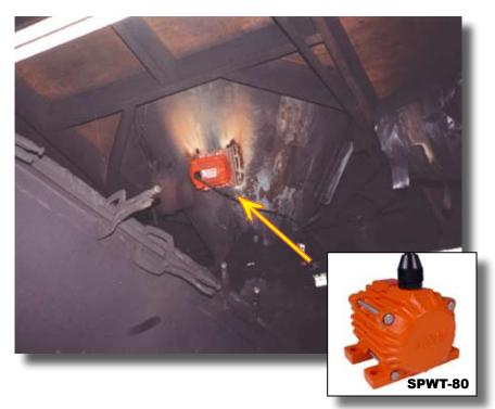
A rice processing company was having difficulty moving their burned rice hulls (ash) out of the hopper into the auger. The material was bridging in the cone of the hopper, causing blockage at the spout. Employees had to stop their work and bang on the sides of the hopper with a hammer, which was slowing down production and damaging the hopper.
